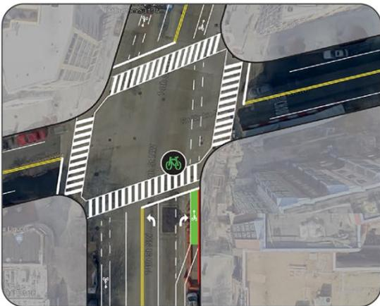
Figure 2c: Through bicycle and vehicle right turn lane, green paint and through intersection guidelines, no mixing zone, bicycle signal and phase separation from right turning vehicles.
