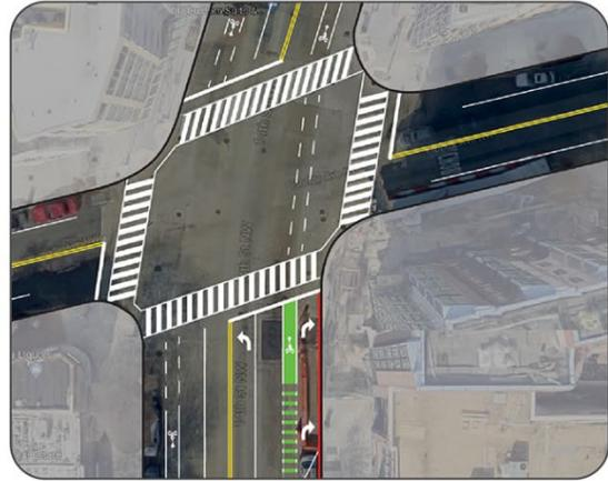
Figure 2b: Through bicycle and vehicle right turn lane with mixing zone, green paint and through intersection guidelines, no physical separation.
