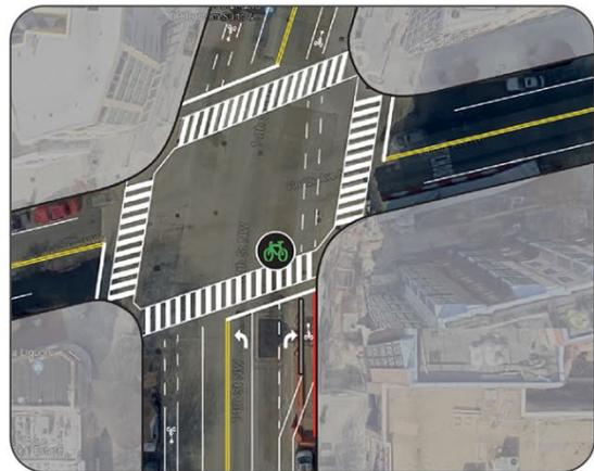
Figure 2d: Through bicycle and vehicle right turn lane, through intersection guidelines, no mixing zone, bicycle signal and phase separation/concrete median separation from right turning vehicles.
