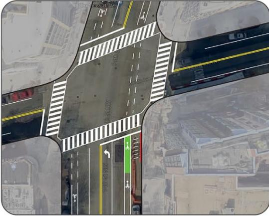
Figure 2a: Through bicycle and vehicle travel lanes, green paint and through intersection guidelines, no physical separation.
