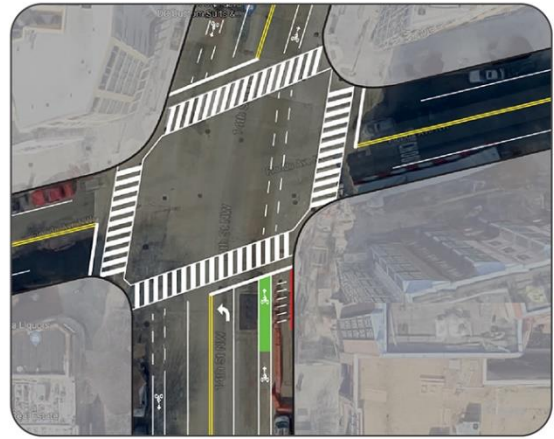
Figure 2a: Through bicycle and vehicle travel lanes, green paint and through intersection guidelines, no physical separation.
