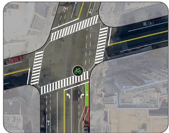
Figure 2c: Through bicycle and vehicle right turn lane, green paint and through intersection guidelines, no mixing zone, bicycle signal and phase separation from right turning vehicles.
